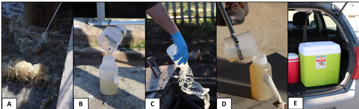
Figure 2: Wastewater grab sampling. A) Collect wastewater with the grab sampling device, after rinsing in the wastewater. B) Pour into the labelled sample bottle, avoid contaminating the outside of the bottle. C) Rinse the inside of the sample bottle with the wastewater and discard of the contents. D) Repeat steps A&B and fill the sample bottle to the brim and close the lid tightly. E) Spray down the sample bottle with 70% ethanol and transport
