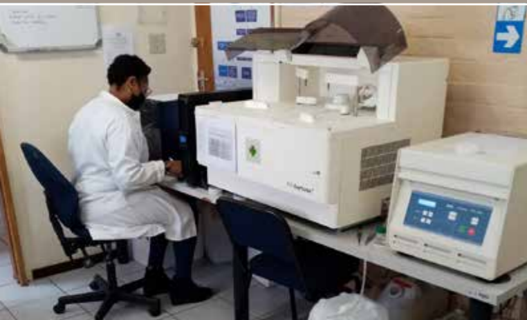
This is the "RX Daytona+" analyser used for analysis of Glucose, Lipids, Albumin, Creatinine
